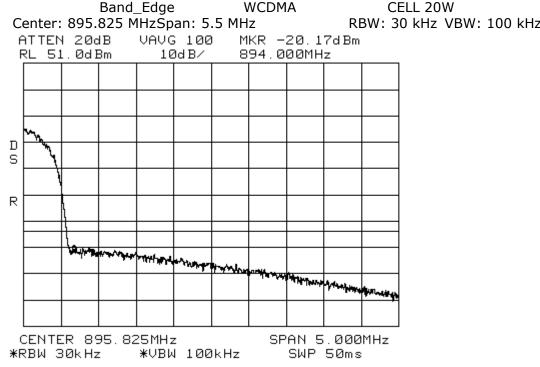
Correction Factor 10log(RBW Needed / RBW Used)  $10\log(50kHz / 30kHz) = 2.2$ Actual = -17.97dB
