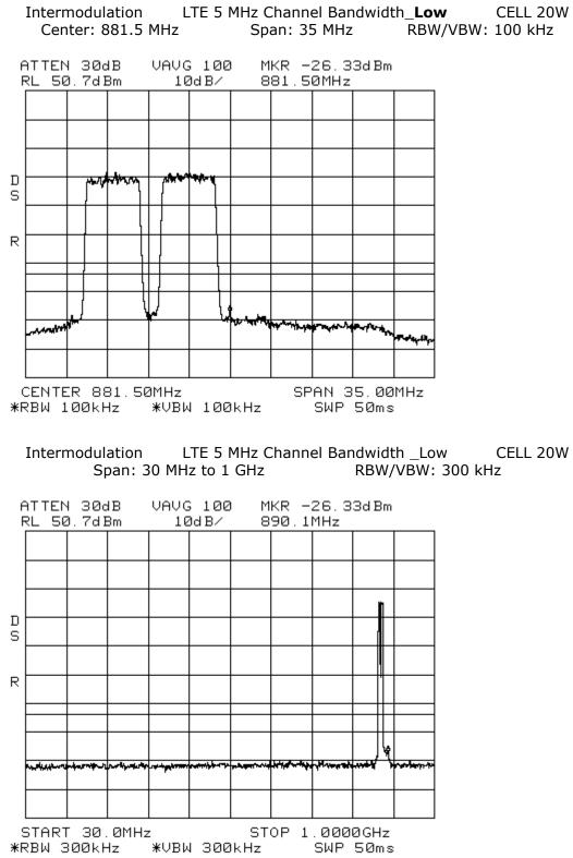
Intermodulation LTE 5 MHz Channel Bandwidth Low CELL 20W
