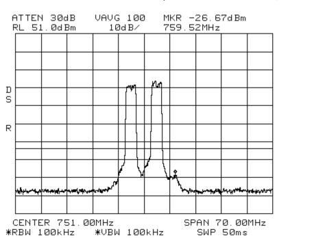
Intermodulation LTE 3 MHz Channel Bandwidth \_Apart 700UpperC Path 2 Center: 751 MHz Span: 70 MHz RBW/VBW: 100 kHz
