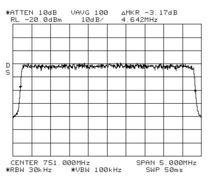
Occupied Bandwidth LTE 5 MHz Channel Bandwidth\_Signal\_In 700UpperC Path 2 Span: 5 MHz RBW: 30 kHz VBW: 100 kHz
