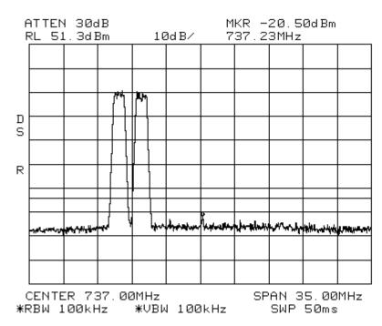
Intermodulation LTE 1.4 MHz Channel Bandwidth \_Low 700LowerABC Span: 30 MHz to 1 GHz RBW/VBW: 300 kHz
