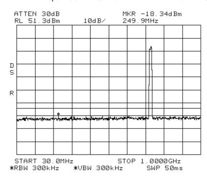
Conducted Emissions LTE 15 MHz Channel Bandwidth 700LowerABC
