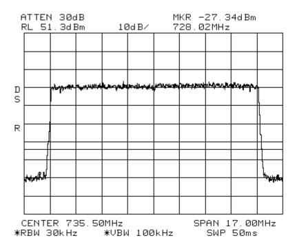
Band\_Edge LTE 15 MHz Channel Bandwidth 700LowerABC Center: 738.5 MHz Span: 17 MHz RBW: 30 kHz VBW: 100 kHz
