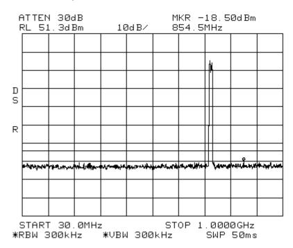
Intermodulation LTE 5 MHz Channel Bandwidth \_Low 700LowerABC
