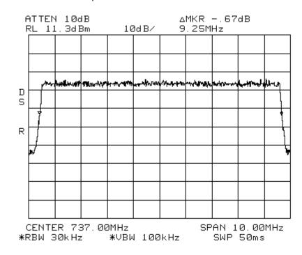
Occupied Bandwidth LTE 10 MHz Channel Bandwidth \_Signal\_Out 700LowerABC
