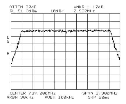
Occupied Bandwidth LTE 5 MHz Channel Bandwidth\_Signal\_In 700LowerABC Span: 5 MHz RBW: 30 kHz VBW: 100 kHz
