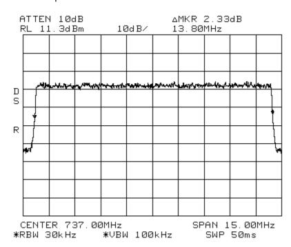
Occupied Bandwidth LTE 15 MHz Channel Bandwidth \_Signal\_Out Span: 15 MHz RBW: 30 kHz VBW: 100 kHz
