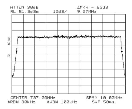
Occupied Bandwidth LTE 15 MHz Channel Bandwidth\_Signal\_In Span: 15 MHz RBW: 30 kHz VBW: 100 kHz
