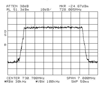
Band\_Edge LTE 5 MHz Channel Bandwidth 700LowerABC Center: 743.3 MHz Span: 7 MHz RBW: 30 kHz VBW: 100 kHz
