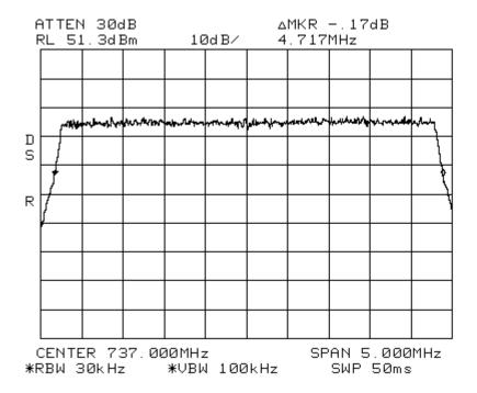
Occupied Bandwidth LTE 10 MHz Channel Bandwidth\_Signal\_In 700LowerABC Span: 10 MHz RBW: 30 kHz VBW: 100 kHz
