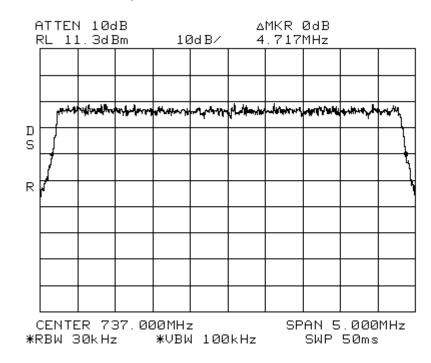
Occupied Bandwidth LTE 5 MHz Channel Bandwidth \_Signal\_Out 700LowerABC
