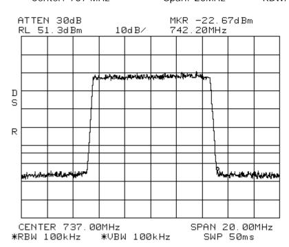
Conducted Emissions LTE 10 MHz Channel Bandwidth 700LowerABC
