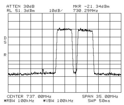
Intermodulation LTE 5 MHz Channel Bandwidth \_High 700LowerABC Span: 30 MHz to 1 GHz RBW/VBW: 300 kHz
