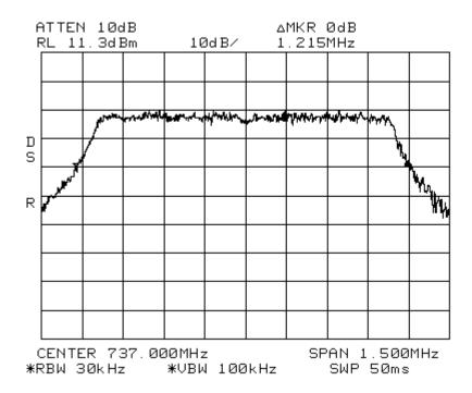
Occupied Bandwidth LTE 1.4 MHz Channel Bandwidth \_Signal\_Out 700LowerABC Span: 1.50 MHz RBW: 30 kHz VBW: 100 kHz
