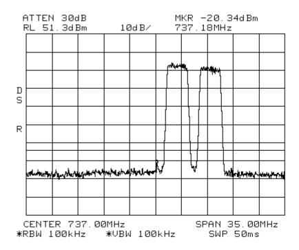
Intermodulation LTE 3 MHz Channel Bandwidth \_High 700LowerABC Span: 30 MHz to 1 GHz RBW/VBW: 300 kHz
