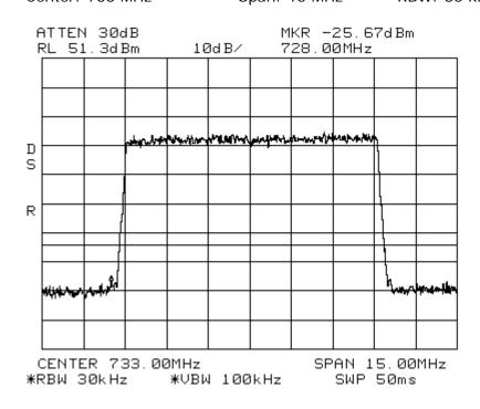
Band\_Edge LTE 10 MHz Channel Bandwidth 700LowerABC Center: 741 MHz Span: 15 MHz RBW: 30 kHz VBW: 100 kHz
