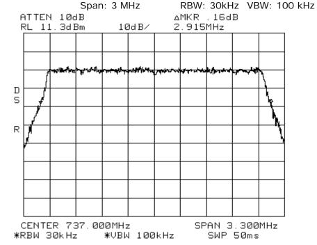
Occupied Bandwidth LTE 3 MHz Channel Bandwidth \_Signal\_Out 700LowerABC Span: 3 MHz RBW: 30 kHz VBW: 100 kHz
