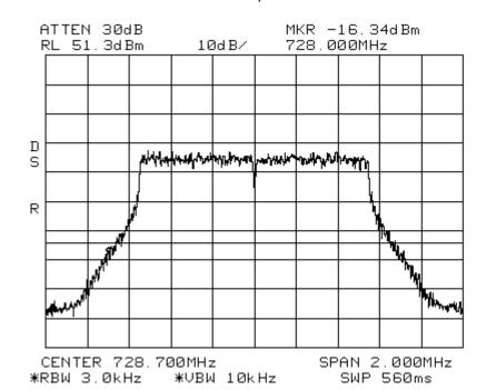
Band\_Edge LTE 1.4 MHz Channel Bandwidth 700LowerABC Center: 745.3 MHz Span: 2 MHz RBW: 3 kHz VBW: 10 kHz
