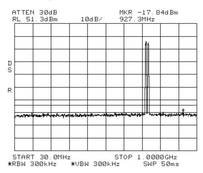
Intermodulation LTE 5 MHz Channel Bandwidth \_Apart 700LowerABC
