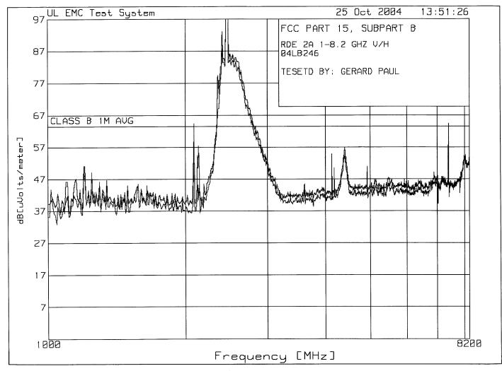
Note: Emission shown on plot from 2.2 GHz to 3.2 GHz represents mathematical correction for band reject filter used for test plus some emissions at transmit frequency. Actual emissions at 2.4 to 2.4835 GHz are determined from conducted power measurements.
