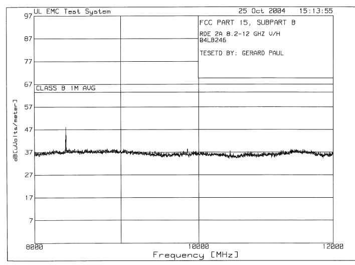
Note: Measurement performed at 1 meter distance with General Limit adjusted by 20\*log(3m/1m) dB, or 9.5 dB.
