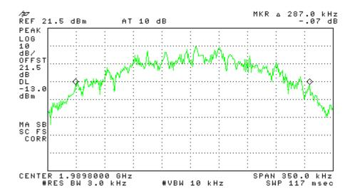
Occupied Bandwidth Span: 350 kHz EDGE\_Signal\_Out RBW: 3 kHz VBW: 10 kHz
