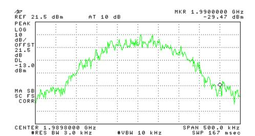
Band\_Edge Center: 1930.2 MHz Span: 500 kHz **EDGE**
