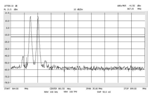
EDGE\_Low CELLULAR Intermodulation Span: 30 MHz to 1 GHz RBW/VBW: 300 kHz
