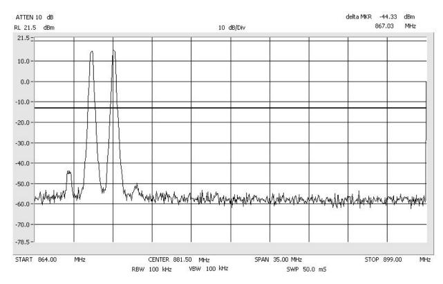
Intermodulation GSM\_Low CELLULAR Span: 30 MHz to 1 GHz RBW/VBW: 300 kHz
