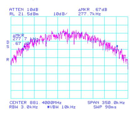
Occupied Bandwidth EDGE\_Signal\_Out RBW: 3 kHz VBW: 10 kHz Span: 350 kHz
