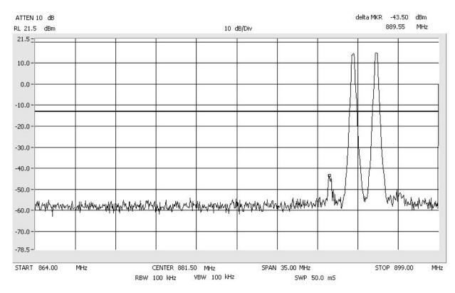
Intermodulation GSM\_High CELLULAR Span: 30 MHz to 1 GHz RBW/VBW: 300 kHz
