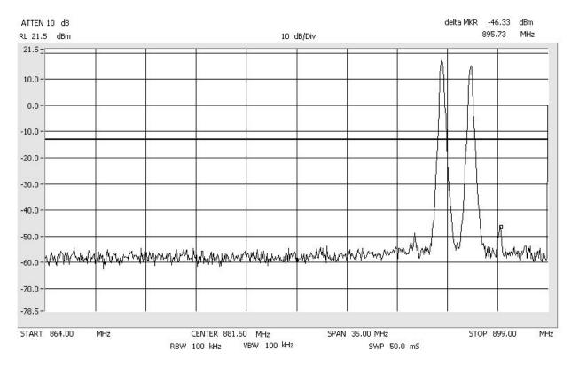
Intermodulation EDGE\_High CELLULAR Span: 30 MHz to 1 GHz RBW/VBW: 300 kHz
