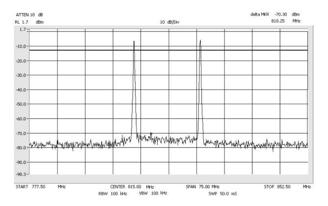
Intermodulation FM\_Apart SMR\_800\_MHz Span: 30 MHz to 1 GHz RBW/VBW: 300 kHz
