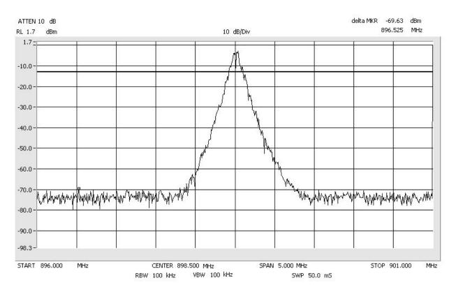
Conducted Emissions iDEN SMR\_900\_MHz Span: 30 MHz to 1 GHz RBW/VBW: 300 kHz
