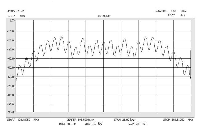
Occupied Bandwidth FM\_Signal\_Out Span: 25 kHz RBW: 300 Hz VBW: 1 kHz
