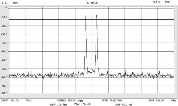
Intermodulation FM\_Apart SMR\_800\_MHz RBW/VBW: 300 kHz Span: 30 MHz to 1 GHz
