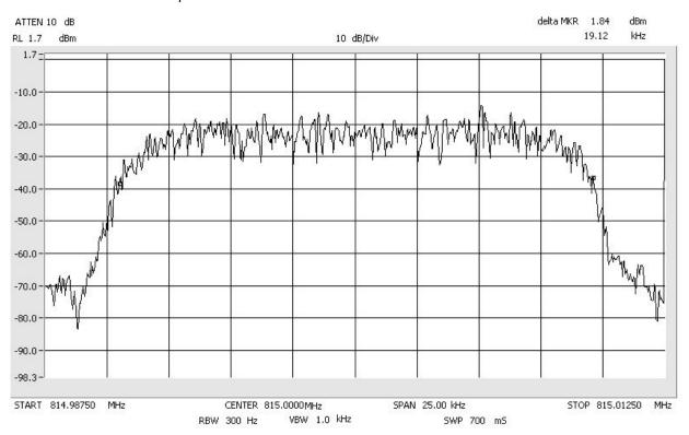
Occupied Bandwidth FM\_Signal\_In Span: 25 kHz RBW: 300 Hz VBW: 1 kHz
