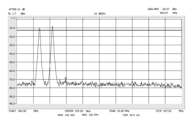
Intermodulation iDEN\_Low SMR\_800\_MHz Span: 30 MHz to 1 GHz RBW/VBW: 300 kHz
