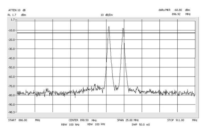
Intermodulation FM\_High SMR\_800\_MHz Span: 30 MHz to 1 GHz RBW/VBW: 300 kHz
