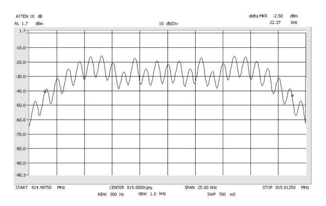
Occupied Bandwidth FM\_Signal\_Out Span: 25 kHz RBW: 300 Hz VBW: 1 kHz
