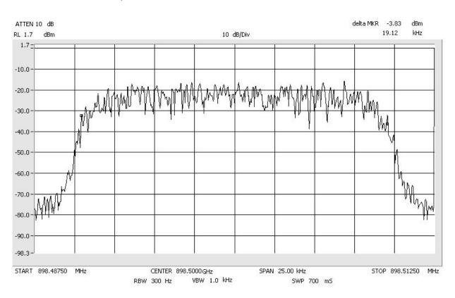
Occupied Bandwidth iDEN\_Signal\_Out Span: 25 kHz RBW: 300 Hz VBW: 1 kHz
