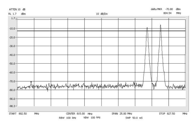
Intermodulation iDEN\_High SMR\_800\_MHz Span: 30 MHz to 1 GHz RBW/VBW: 300 kHz
