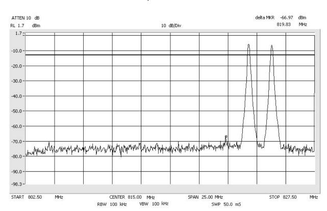
Intermodulation SMR\_800\_MHz FM\_High Span: 30 MHz to 1 GHz RBW/VBW: 300 kHz
