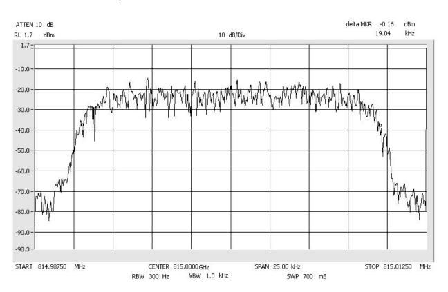
Occupied Bandwidth iDEN\_Signal\_Out Span: 25 kHz RBW: 300 Hz VBW: 1 kHz
