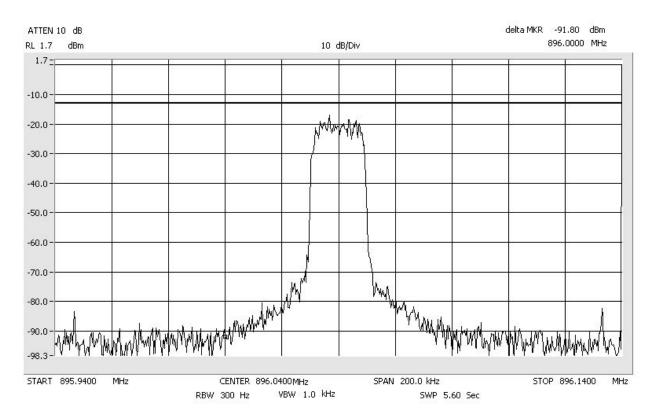
Band\_Edge iDEN Center: 900.92 MHz Span: 200 kHz RBW: 300 Hz VBW: 1 kHz
