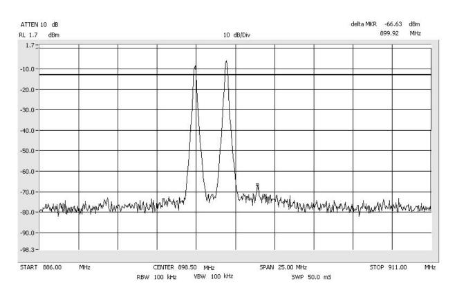
Intermodulation FM\_Low SMR\_900\_MHz Span: 30 MHz to 1 GHz RBW/VBW: 300 kHz
