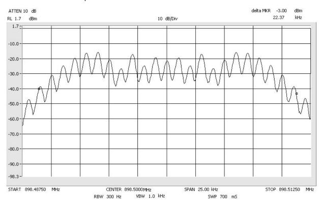
Occupied Bandwidth iDEN\_Signal\_In Span: 25 kHz RBW: 300 Hz VBW: 1 kHz
