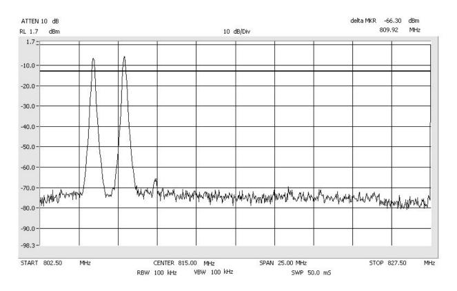
Intermodulation FM\_Low SMR\_800\_MHz Span: 30 MHz to 1 GHz RBW/VBW: 300 kHz
