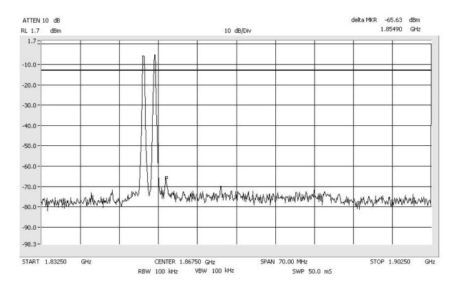
Intermodulation\_LowGSM\_Low PCS Span: 30 MHz to 1 GHz RBW/VBW: 300 kHz
