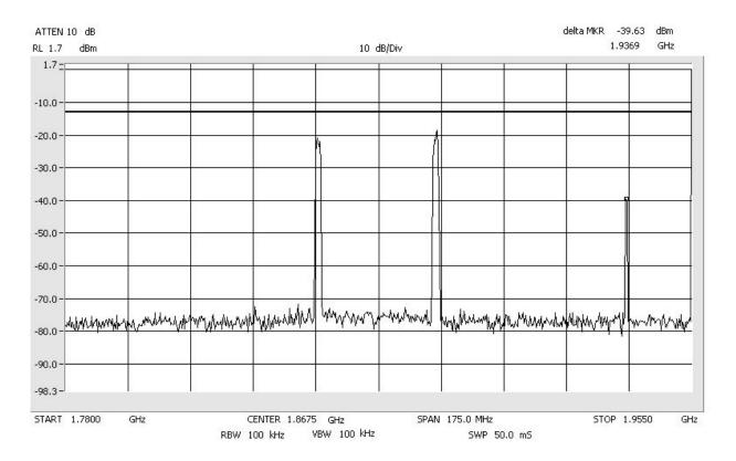
Intermodulation\_LowCDMA\_Apart PCS Span: 30 MHz to 1 GHz RBW/VBW: 300 kHz
