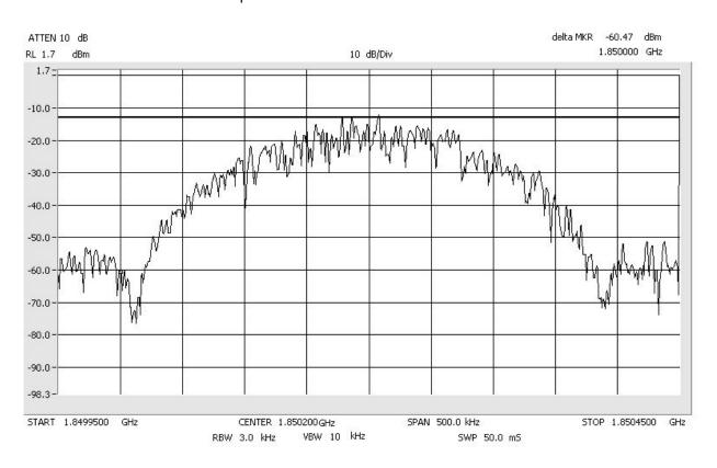
Band\_Edge EDGE Center: 1909.8 MHz Span: 500 kHz RBW: 3 kHz VBW: 10 kHz
