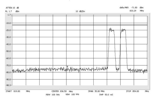
Intermodulation CDMA\_High CELLULAR Span: 30 MHz to 1 GHz RBW/VBW: 300 kHz
