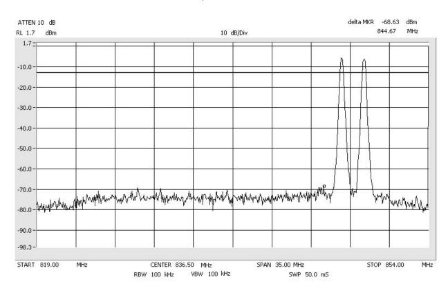
Intermodulation GSM\_High CELLULAR Span: 30 MHz to 1 GHz RBW/VBW: 300 kHz
