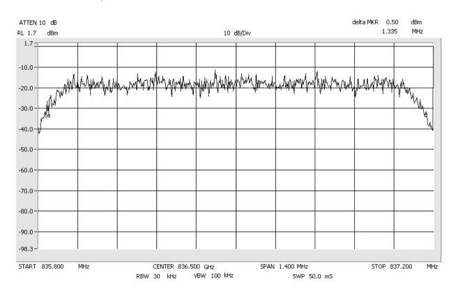
Occupied Bandwidth CDMA\_Signal\_Out Span: 1.4 MHz RBW: 30 kHz VBW: 100 kHz
