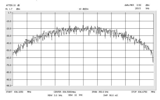
Occupied Bandwidth CDMA\_Signal\_In Span: 1.4 MHz
