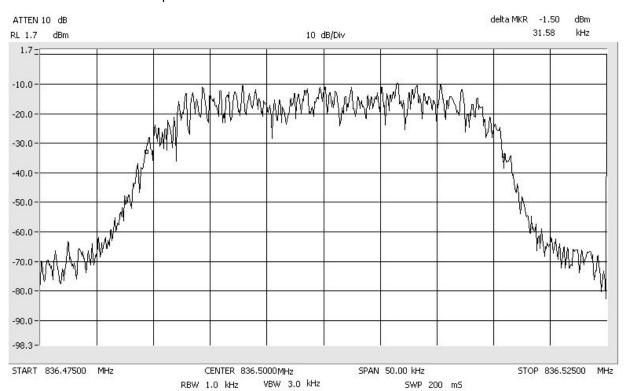
Occupied Bandwidth GSM\_Signal\_In Span: 350 kHz
