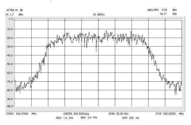
Occupied Bandwidth TDMA\_Signal\_Out Span: 50 kHz RBW: 1 kHz VBW: 3 kHz
