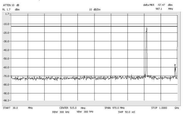
Intermodulation CDMA\_Low CELLULAR Span: 1 GHz to 10 GHz RBW/VBW: 1 MHz
