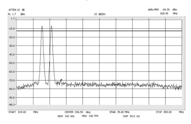
Intermodulation EDGE\_Low CELLULAR Span: 30 MHz to 1 GHz RBW/VBW: 300 kHz
