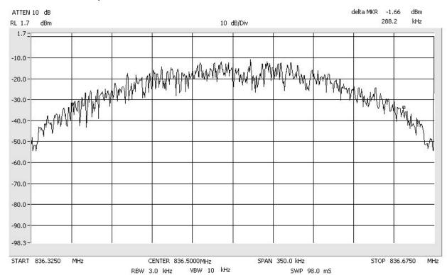
Occupied Bandwidth EDGE\_Signal\_In Span: 350 kHz
