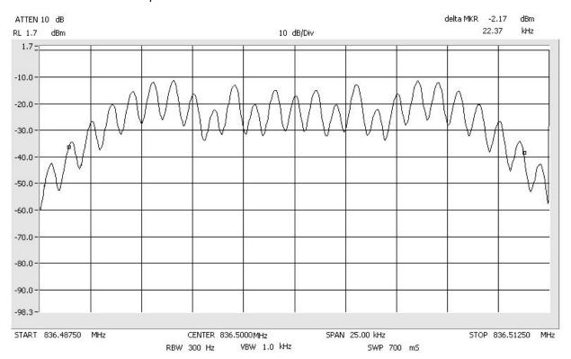
Occupied Bandwidth TDMA\_Signal\_In Span: 50 kHz RBW: 1 kHz VBW: 3 kHz
