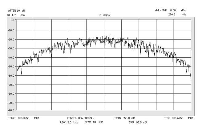
Occupied Bandwidth GSM\_Signal\_Out Span: 350 kHz RBW: 3 kHz VBW: 10 kHz
