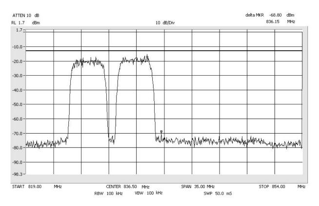
Intermodulation WCDMA\_Low CELLULAR Span: 30 MHz to 1 GHz RBW/VBW: 300 kHz
