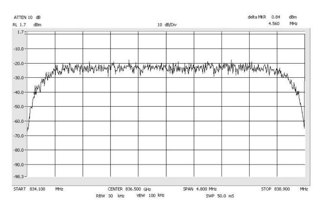
Occupied Bandwidth WCDMA\_Signal\_Out Span: 4.8 MHz RBW: 30 kHz VBW: 100 kHz
