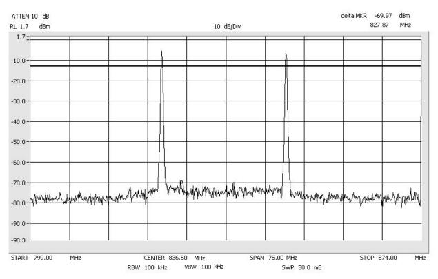
Intermodulation FM\_Apart CELLULAR Span: 30 MHz to 1 GHz RBW/VBW: 300 kHz
