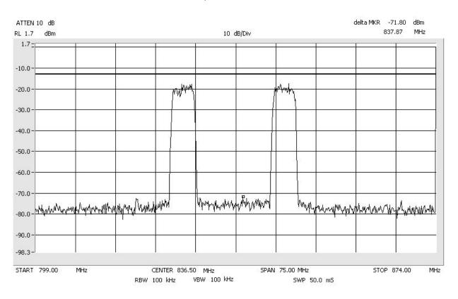
Intermodulation WCDMA\_Apart CELLULAR Span: 30 MHz to 1 GHz RBW/VBW: 300 kHz
