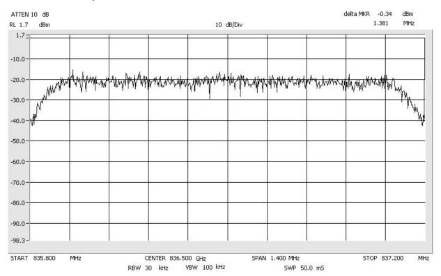
Occupied Bandwidth Span: 4.8 MHz WCDMA\_Signal\_In RBW: 30 kHz VBW: 100 kHz
