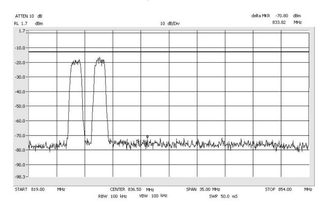
Intermodulation CDMA\_Low CELLULAR Span: 30 MHz to 1 GHz RBW/VBW: 300 kHz
