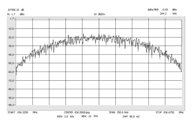
Occupied Bandwidth EDGE\_Signal\_Out Span: 350 kHz RBW: 3 kHz VBW: 10 kHz
