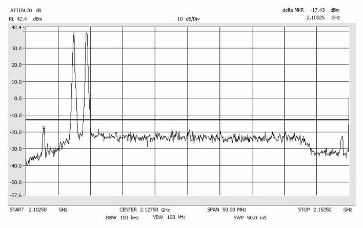
TDMA Lower Band Intermodulation Close - Lower AWS
