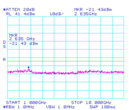
Intermodulation WCDMA\_Apart CELLULAR Span: 1 GHz to 10 GHz RBW/VBW: 1 MHz
