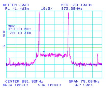
Intermodulation EDGE\_Apart CELLULAR Center: 881.5 MHz Span: 75 MHz RBW/VBW: 100 kHz
