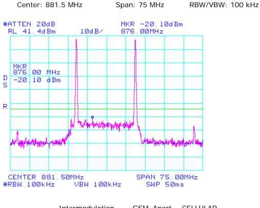
Intermodulation Span: 30 MHz to 1 GHz
