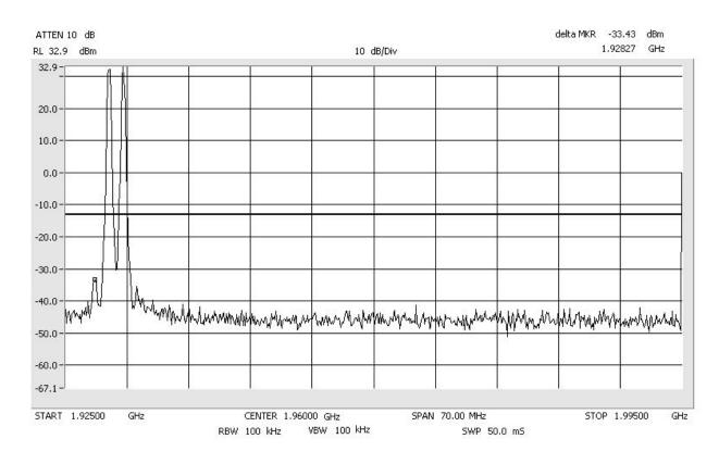
Intermodulation GSM\_Low PCS Span: 30 MHz to 1 GHz RBW/VBW: 300 kHz
