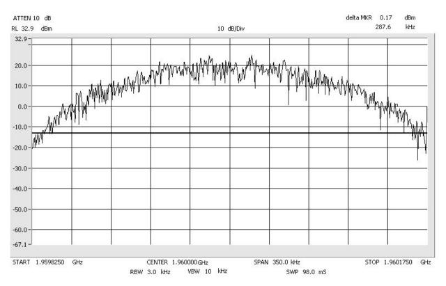
Occupied Bandwidth Span: 350 kHz
