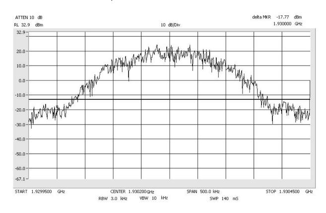
Band\_Edge GSM Center: 1989.8 MHz Span: 500 kHz RBW: 3 kHz VBW: 10 kHz
