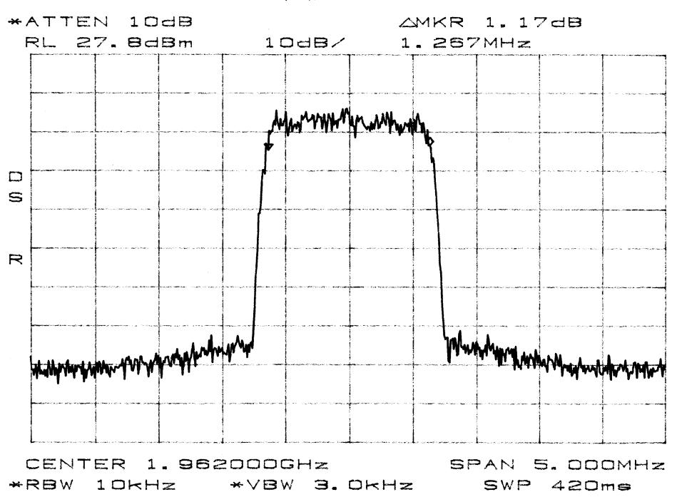
Occupied Band width BAND B,F,F CDMA OUT
