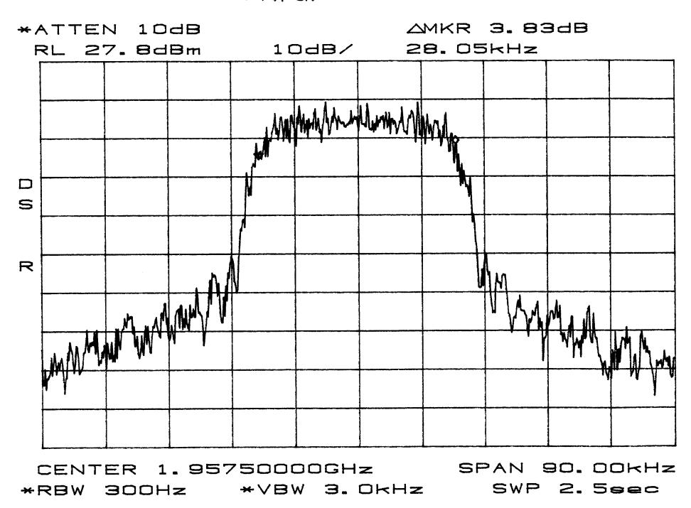
Occupied Band with BAND D, B, E TDMA OUT
