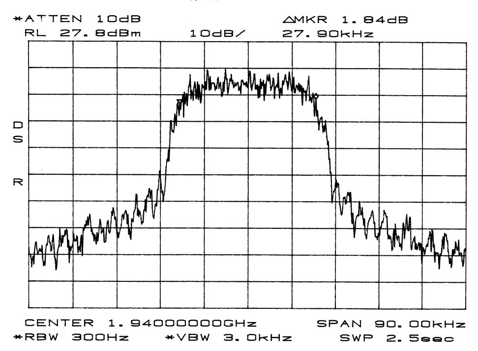
Occupied Band With BAND A,D TDMA OUT
