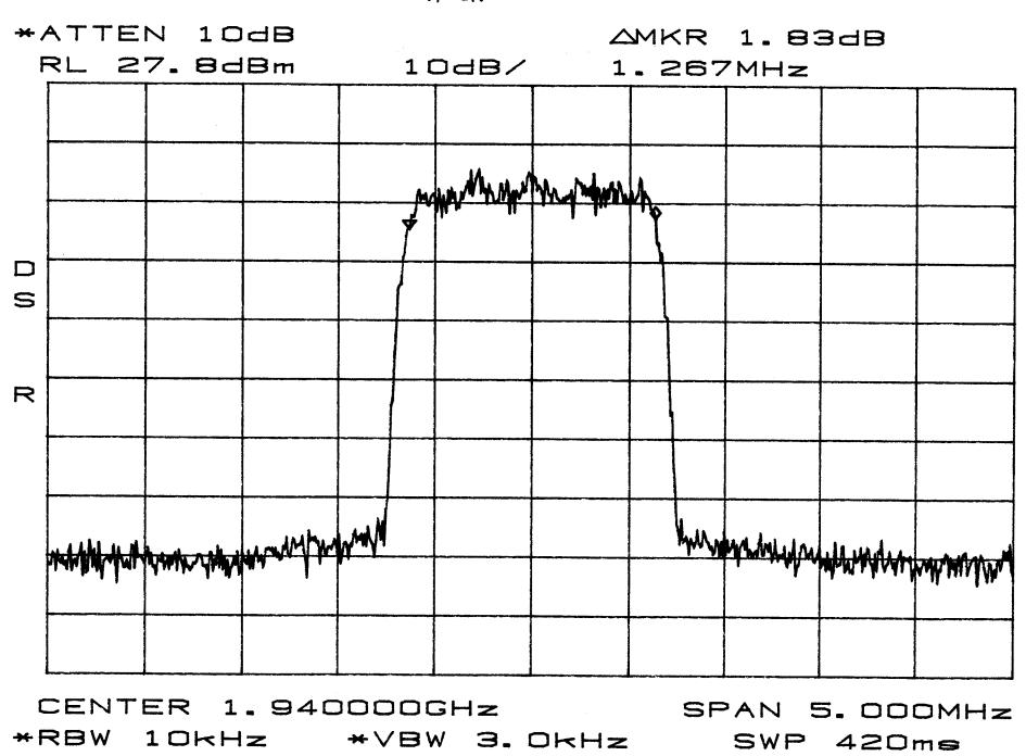
Occupied Band width BAND A, D CDMA OUT
