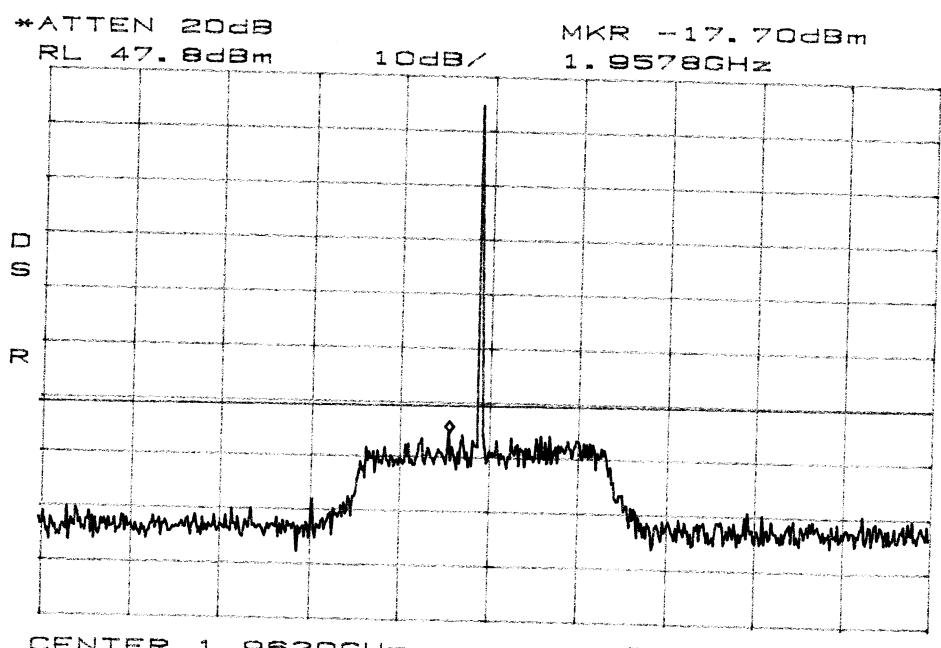
CENTER 1.9620GHz \*RBW 30KHz VBW 30KHz
