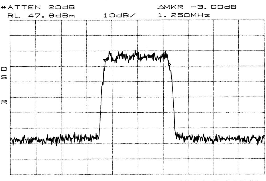
CENTER 1.977000GHz \*RBW 10kHz \*VBW 3.0kHz
