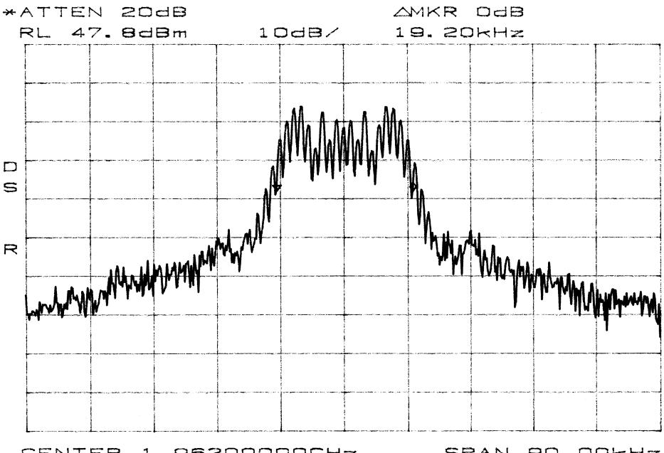
CENTER 1.96200000GHz \*RBW 300Hz \*VBW 3.0KHz SPAN 90. OOKHZ SWP 2. 5sec Occupied Band width BAND B.E, F TDMA IN
