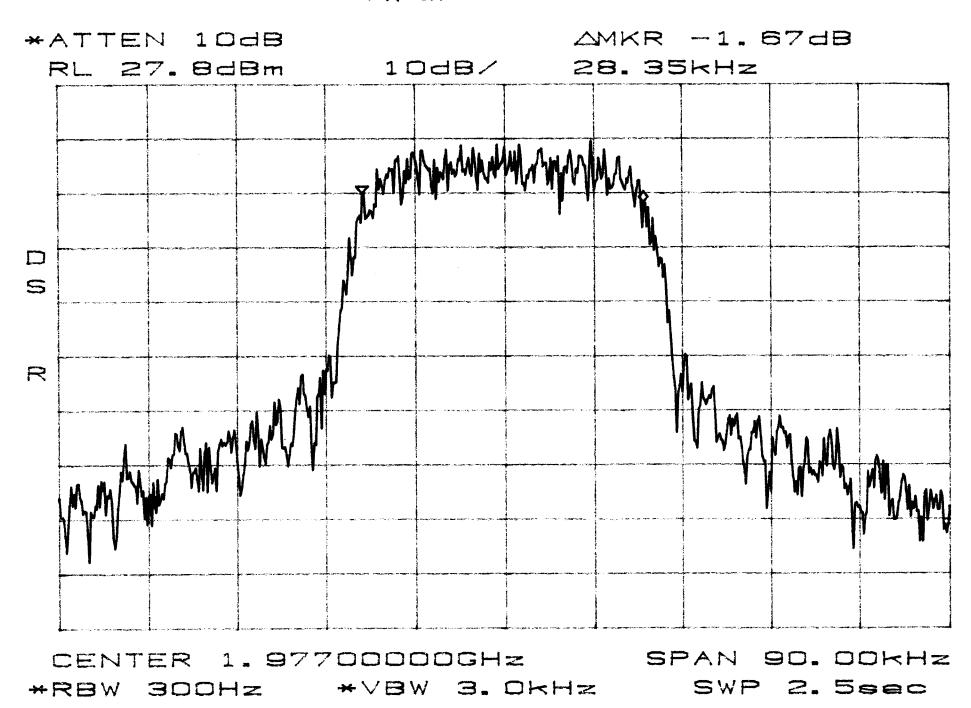
Occupied Band with BAND E,F,C TDMA OUT
