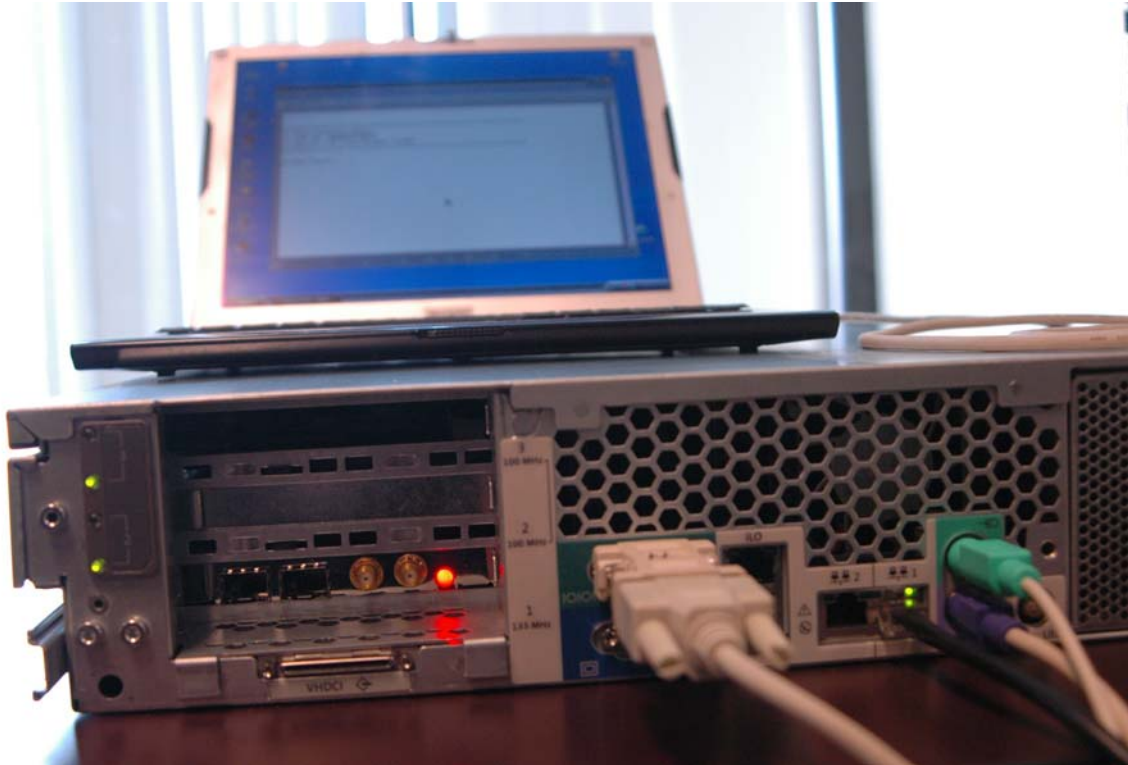
Figure 1: Null modem cable connected to the serial console port of the HP Proliant server
