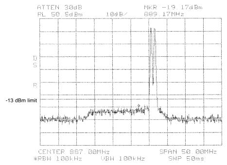
Intermodulation High GSM B BAND
