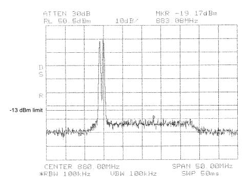
Intermodulation Low GSM A BAND Channel 128 Channel 133
