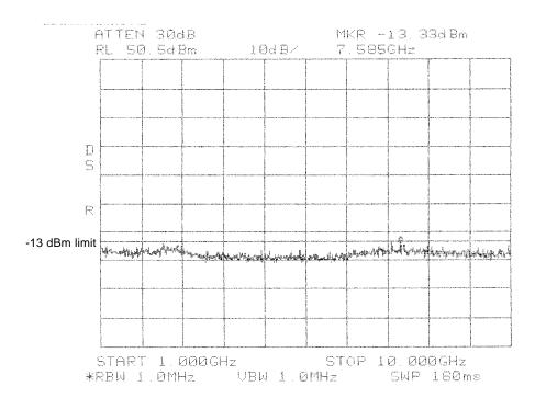
Intermodulation High GSM A BAND
