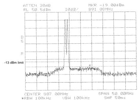
Intermodulation Low GSM B BAND
