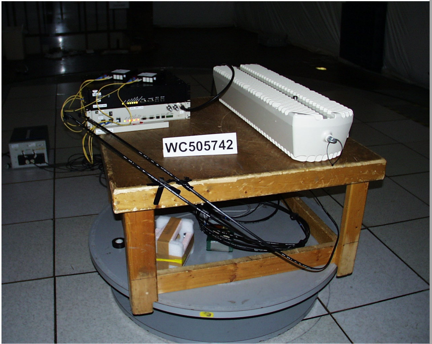
Test setup photo, radiated emissions
