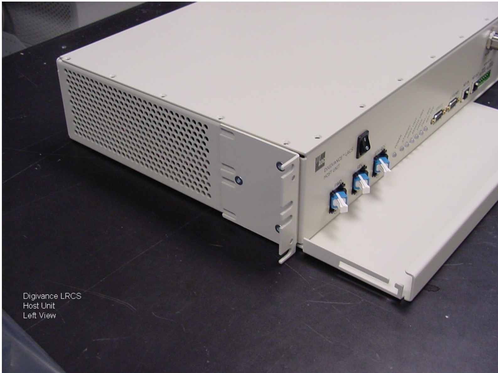
Digivance LRCS 1900 MHz Host Unit Left View
