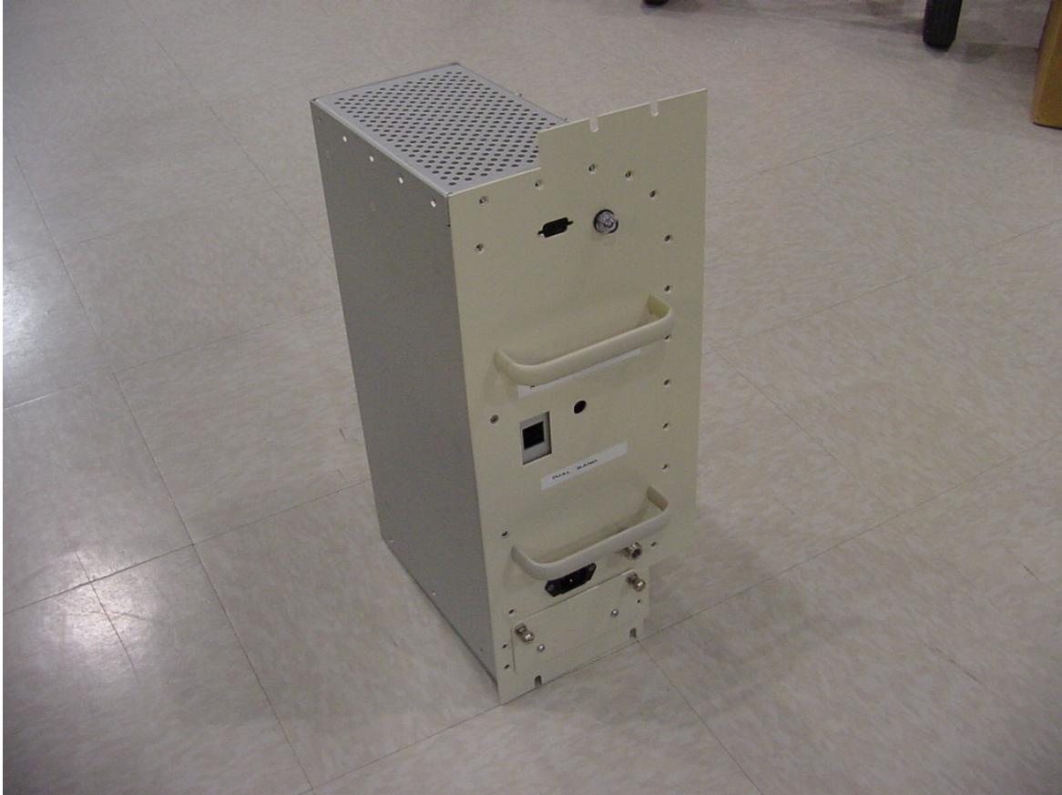
Digivance SCX - SMR Remote Unit Left View
