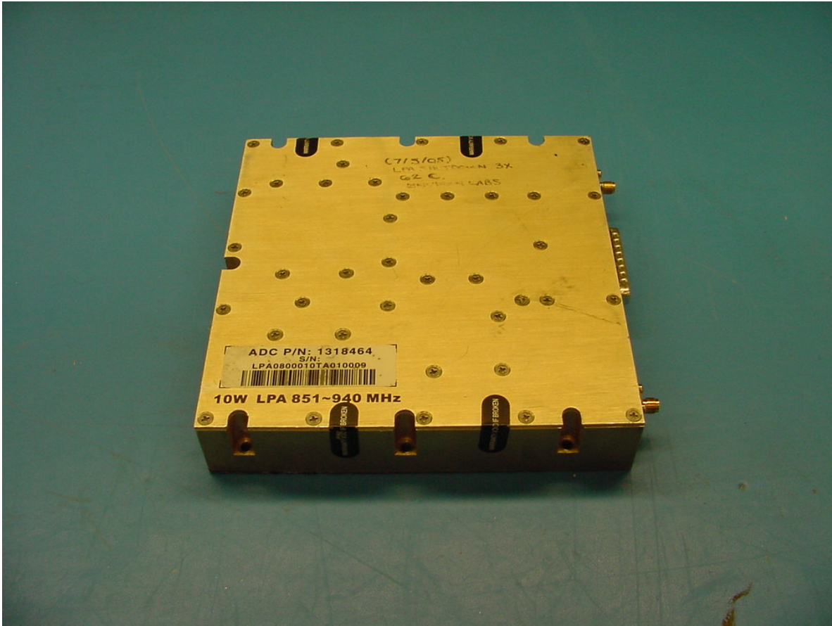
Bravo Tech SMR 800/900 Dual Band Linear Power Amplifier - 10 Watt Front View
