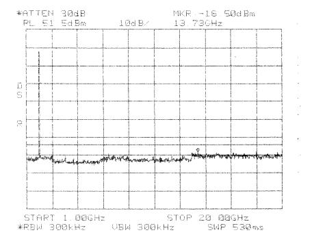
Intermodulation Close Upper TDMA PCS 1900 MHz AD Band
