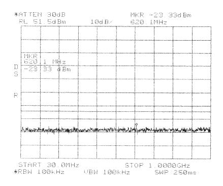
Intermodulation Close Lower TDMA PCS 1900 MHz BEF Band
