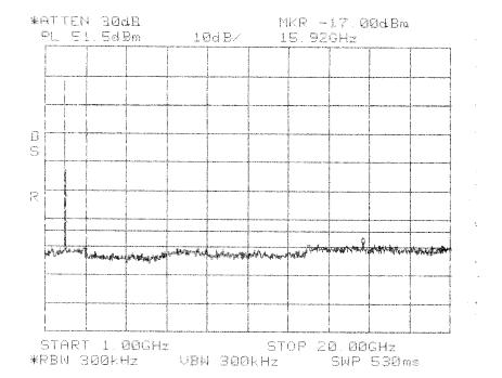
Intermodulation Close Lower GSM PCS 1900 MHz AD Band
