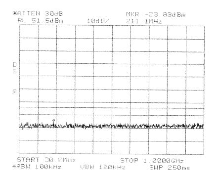
Intermodulation Close Upper TDMA PCS 1900 MHz DBE Band
