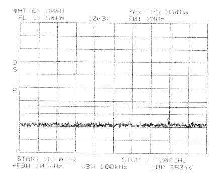
Intermodulation **Apart TDMA PCS 1900 MHz EFC Band**
