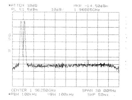
Intermodulation Close Lower GSM PCS 1900 MHz BEF Band
