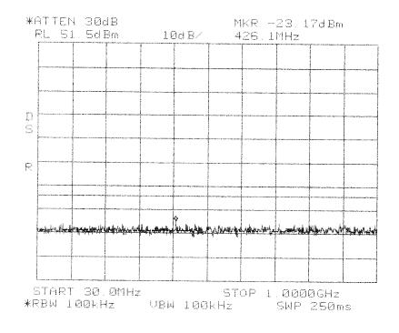
Intermodulation Close Upper TDMA PCS 1900 MHz AD Band
