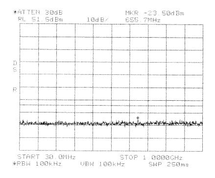
Intermodulation **Apart GSM PCS 1900 MHz BEF Band**
