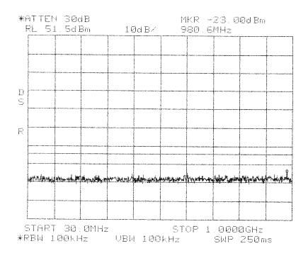
Intermodulation Close Lower **TDMA PCS 1900 MHz AD Band**
