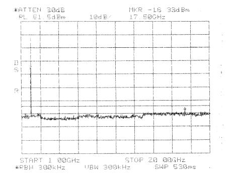
Intermodulation Apart TDMA PCS 1900 MHz AD Band
