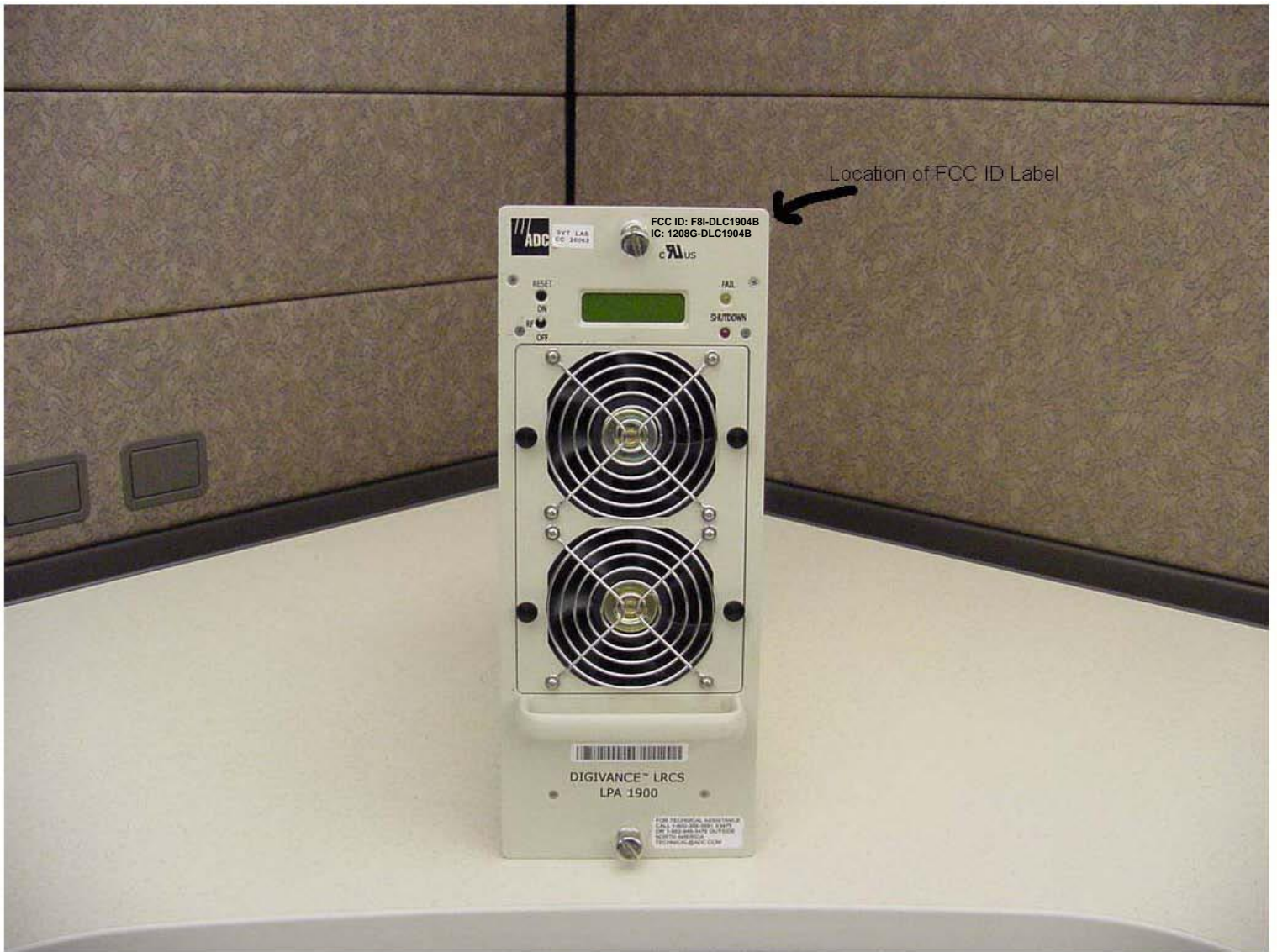
1900 MHz Linear Power Amplifier Location of FCC/IC ID Label
