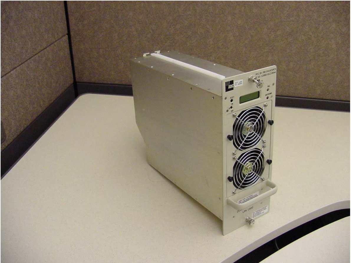
1900 MHz Linear Power Amplifier Left View
