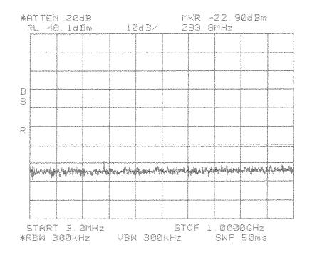
Intermodulation Apart TDMA PCS 1900 MHz AD Band
