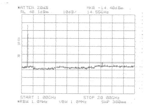
Intermodulation Close Upper TDMA PCS 1900 MHz DBE Band
