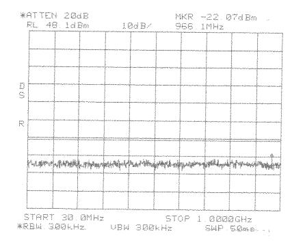
Intermodulation Close Upper TDMA PCS 1900 MHz BEF Band
