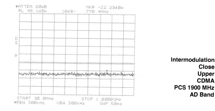
Span: 30 MHz to 1 GHz RBW/VBW: 300 kHz
