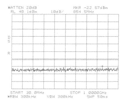
Intermodulation Close Lower GSM PCS 1900 MHz AD Band
