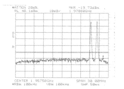
Intermodulation Close Upper TDMA PCS 1900 MHz DBE Band
