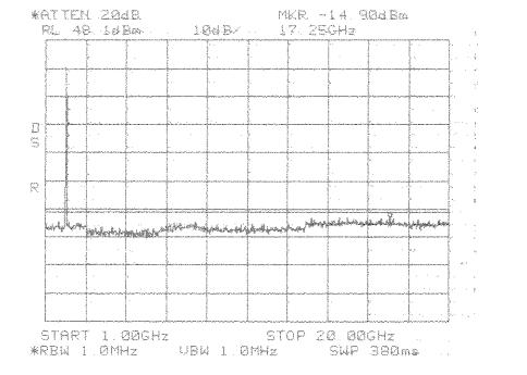
Intermodulation Close Upper TDMA PCS 1900 MHz BEF Band
