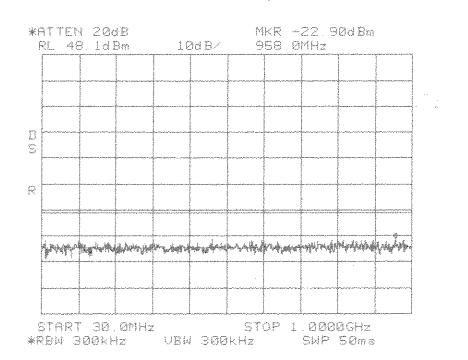
Intermodulation Close Lower TDMA PCS 1900 MHz BEF Band
