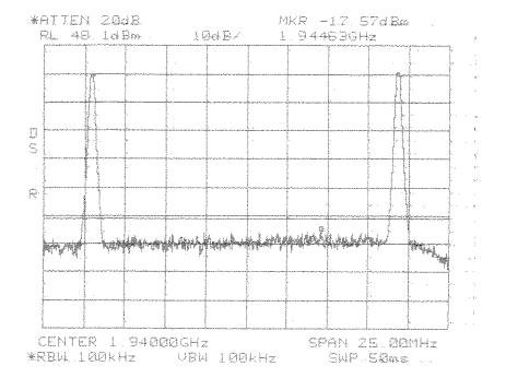
Intermodulation Apart GSM PCS 1900 MHz AD Band
