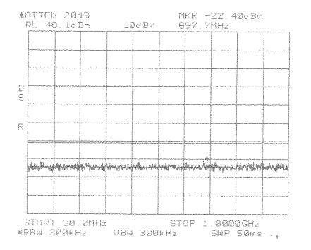
Intermodulation Close Lower TDMA PCS 1900 MHz DBE Band
