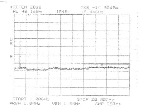
Intermodulation Close Lower GSM PCS 1900 MHz BEF Band
