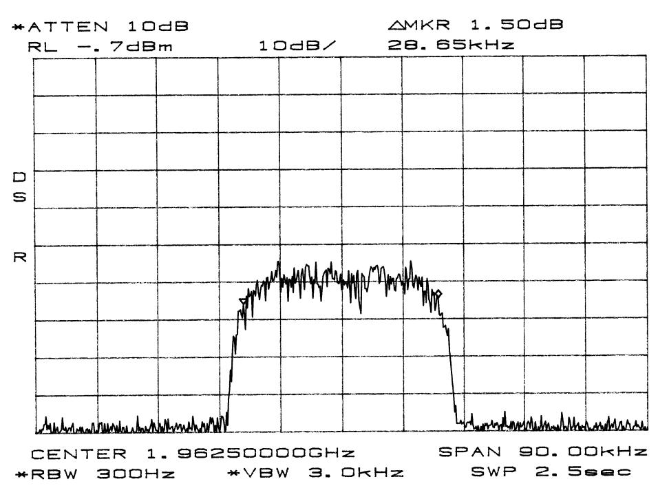
Occupied Band With BAND B, E, F TDMA OUT
