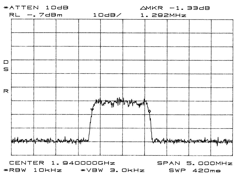
Occupied Band width BAND A,D CDMA OUT
