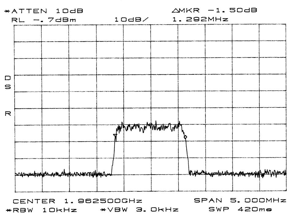
Occupied Band width BAND B, F, F CDMA OUT
