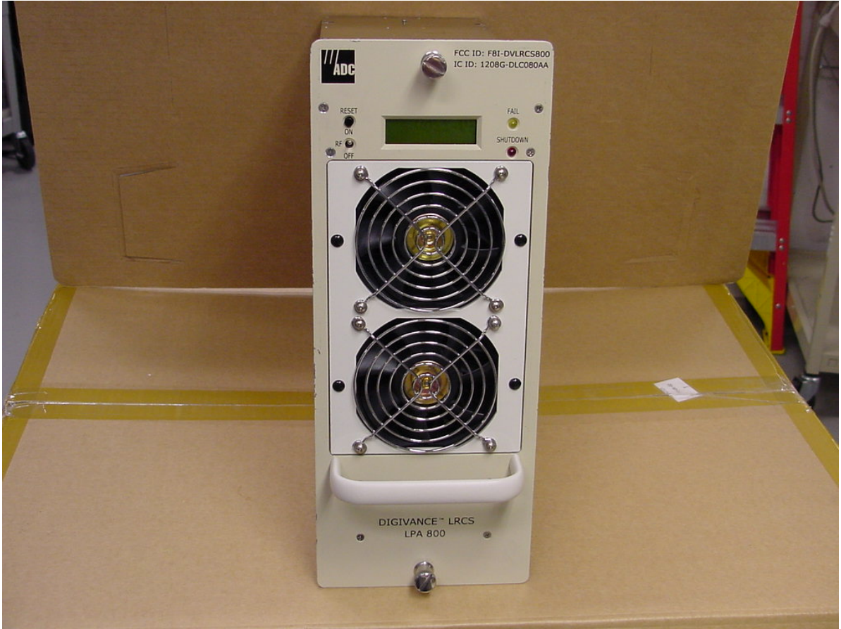
800 MHz Linear Power Amplifier Front View
