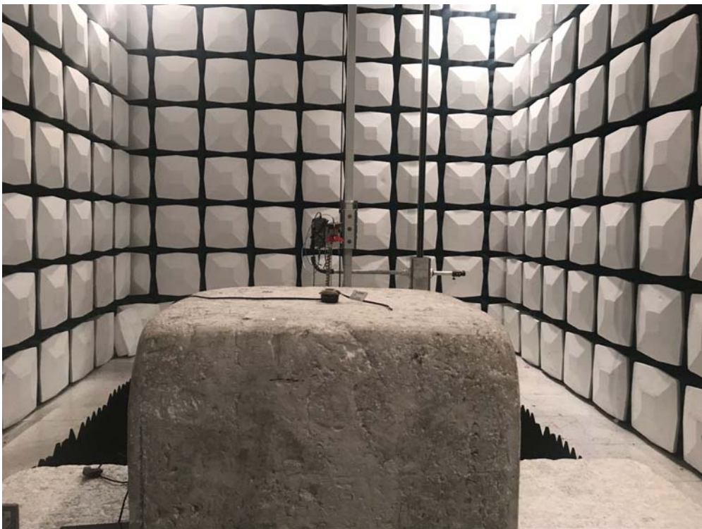
Description: Radiated Emission Test Setup for 1~18GHz
