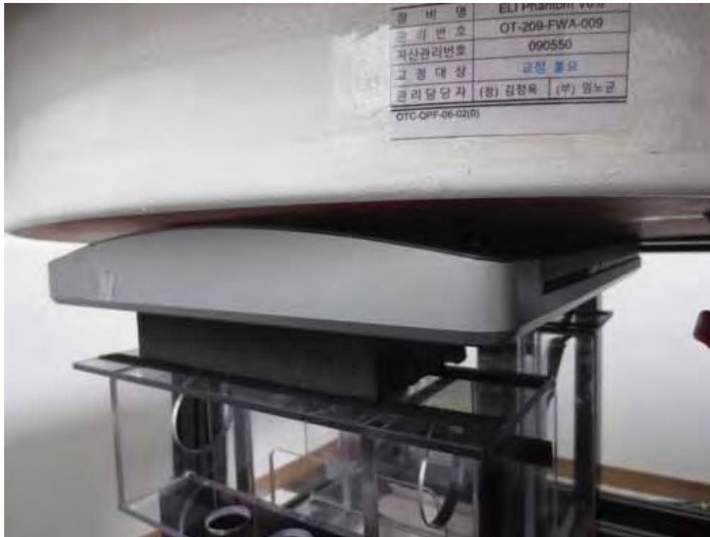
Front from Flat Phantom (Separation Distance: 0 cm)
