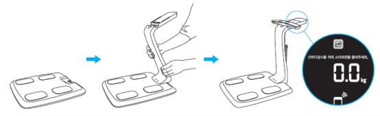
5. Pass the handle's cable through the hole in the rack at the top of the stand and release the handle.
