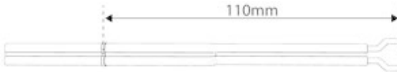
Figure 14: Marking the cable
