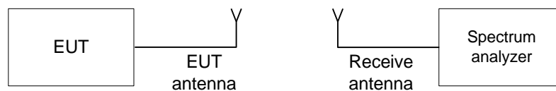
Figure 7.7.1 Band edge emission test setup
