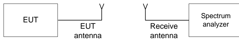
Figure 7.7.1 Band edge emission test setup
