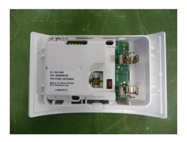
Photograph No.3 Glass Break Detector PGP9922 P9M3 Component side of the main PCB
