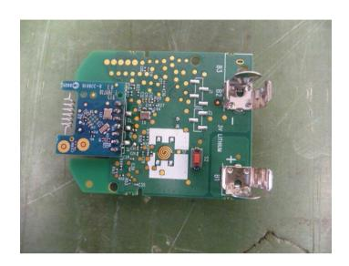
Photograph No.5 Glass Break Detector PGP9922 P9M3 Component side of the RFD board
