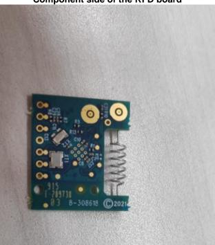
Photograph No.6 Glass Break Detector PGP9922 P9M3 Print side of the RFD board
