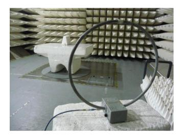
Photograph No.4 Setup for carrier and spurious emissions measurements in anechoic chamber from 30 MHz to 1 GHz
