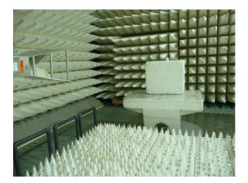
Photograph No.6 Setup for carrier field strength measurements, EUT cabling
