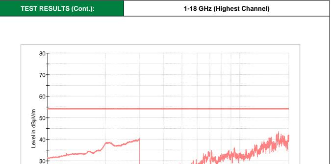
AVG\_MAXH TX limits to Spurious Emission FCC15.249 (Above 1 GHz) 902-928MHz\_Average
