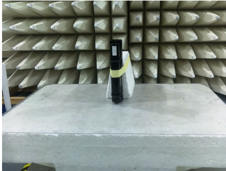
Photograph 8.1.3 Setup for radiated emission measurements, EUT cabling
