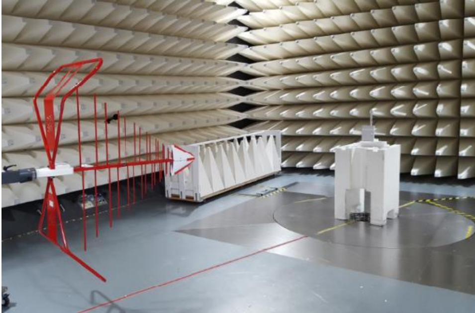
Figure C5. Radiated Emission test setup 1
