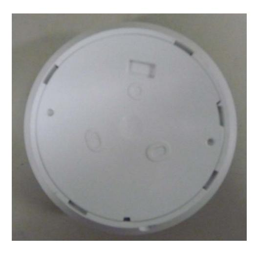
Photograph No.2 PG9862 PIR presence/security detector rear side view
