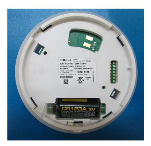
Photograph No.3 PG9862 PIR presence/security rear side view with backplane removed
