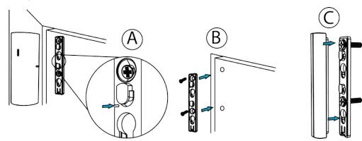
11. **Optional:** You can add 3 mm or 7 mm spacers to the magnet. Clip the spacers onto the bracket in the required combination.
