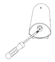
2. Remove the battery while pressing the tamper switch.
