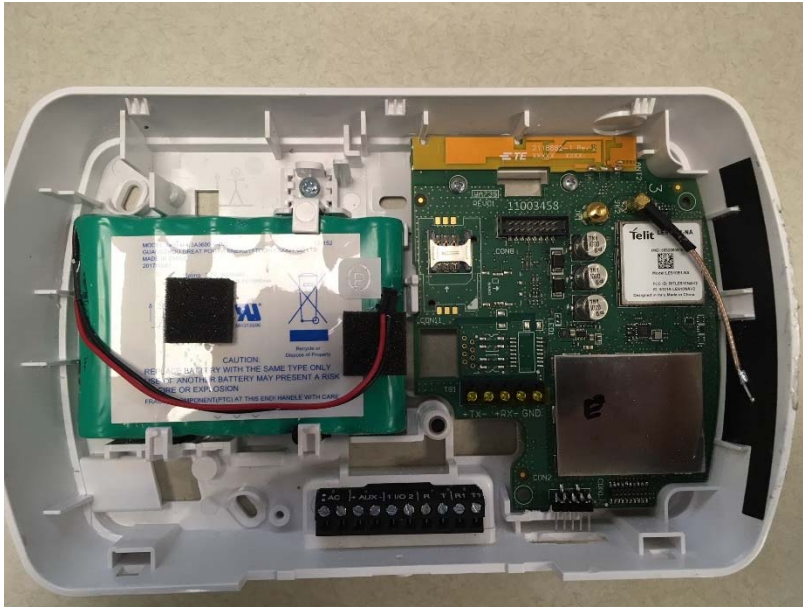
LE2077 (UA735 Rev. 01) PCB top side view (inside the host alarm control panel)
