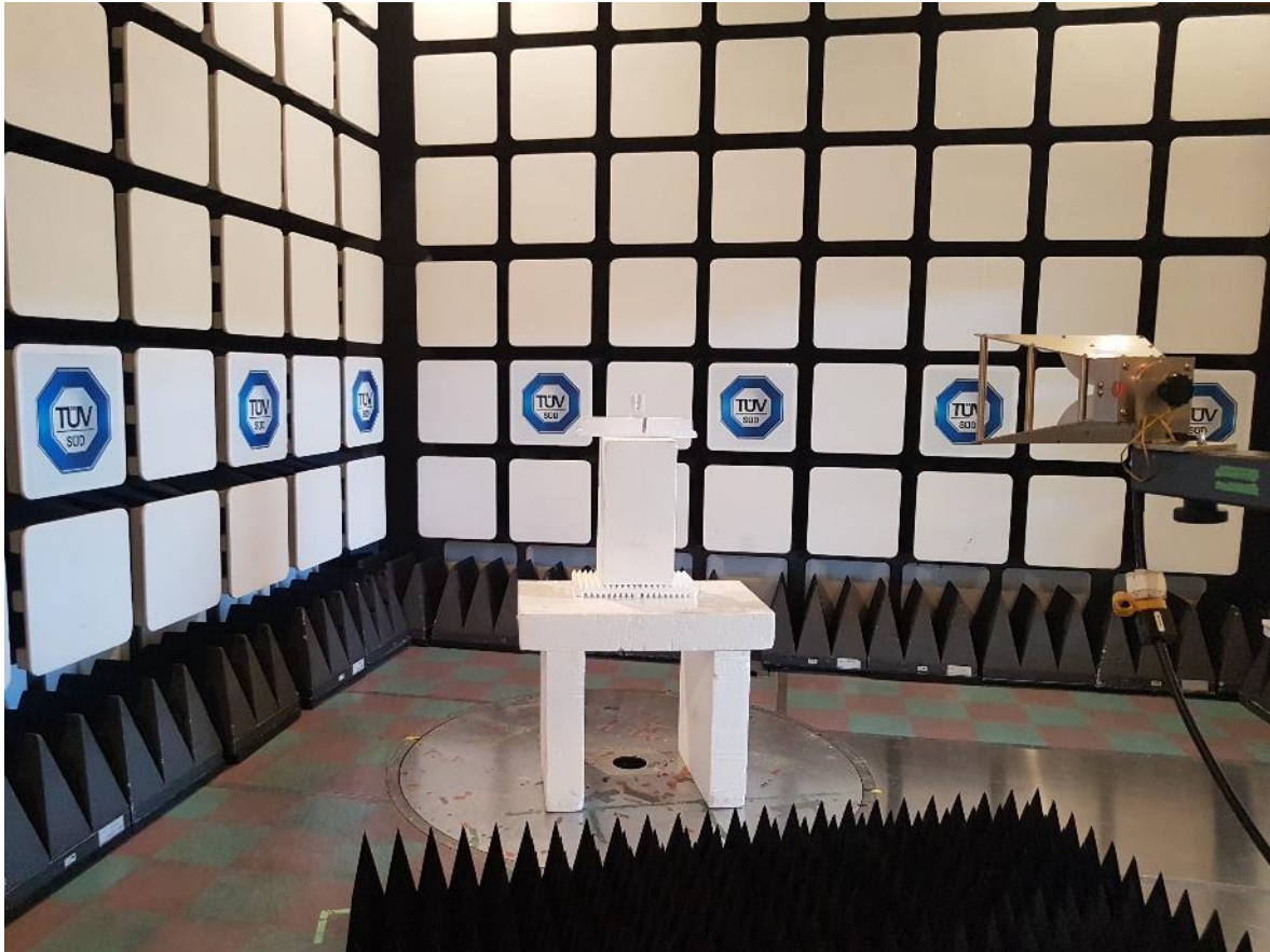
Figure 5 – Radiated Emissions Setup – Photo 4
