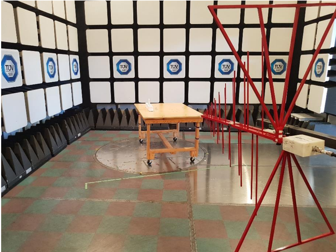
Figure 4 – Radiated Emissions Setup – Photo 3
