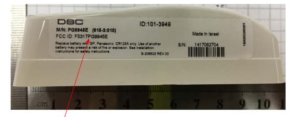
Label with **FCC ID:F5317PG9945E** is located at the side panel. The statement according to FCC part 15 §15.19(a)(3) is placed in User's Guide, page 1 (Application exhibit User\_manual\_29734).
