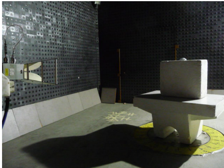
Photograph 8.1.2 Setup for radiated emission measurements above 1 GHz
