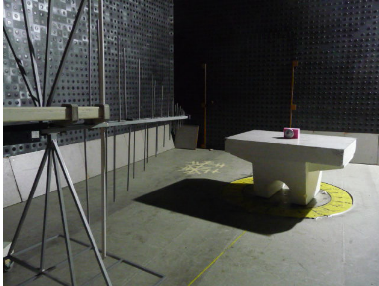
Photograph 8.1.2 Setup for radiated emission measurements above 1 GHz
