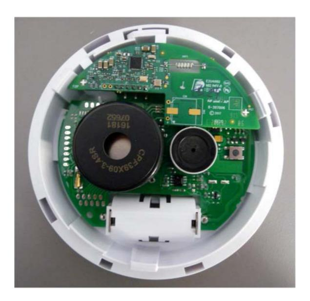
Photograph No.2 Carbon monoxide detector internal view with cover removed
