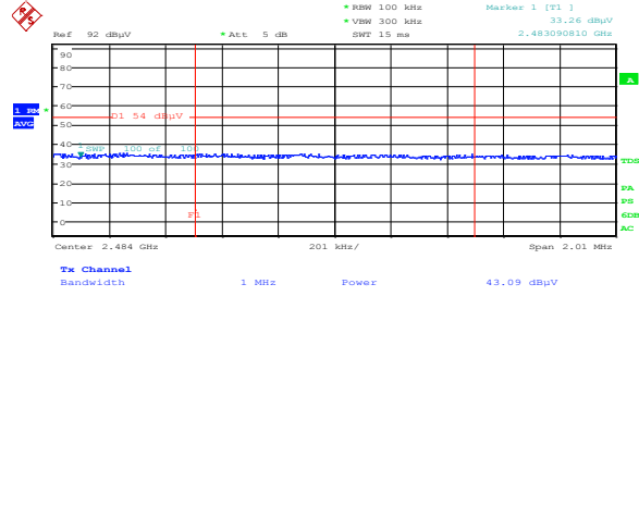
Figure 8.1-20: Radiated spurious emissions Upper band edge for 802.11n HT20, (TX 2462 MHz) – Average
