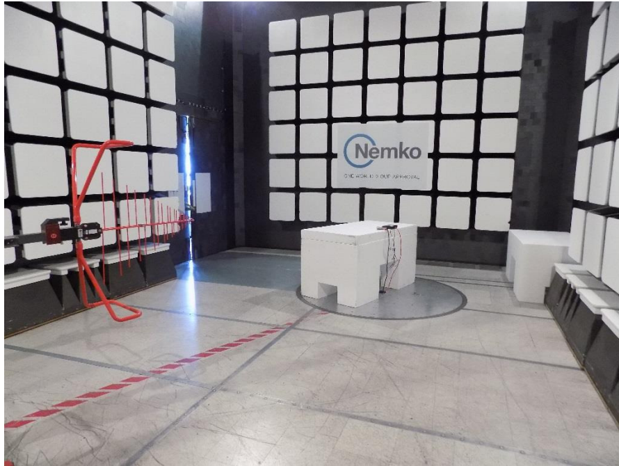
Figure 8.1-29: Radiated spurious (out-of-band) emissions setup photo – 30 to 1000 MHz
