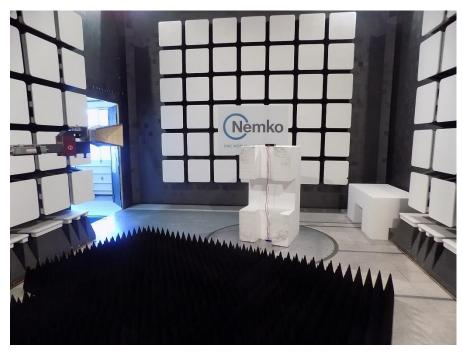
Radiated spurious (out-of-band) emissions setup photo – above 1 GHz
