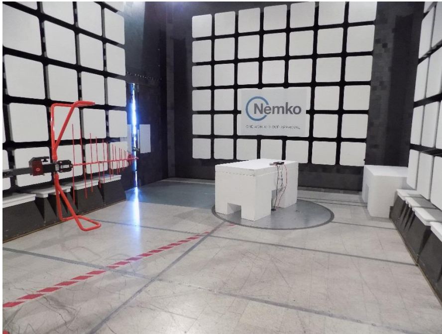
Figure 8.4-58: Radiated spurious (out-of-band) emissions setup photo – 30 to 1000 MHz
