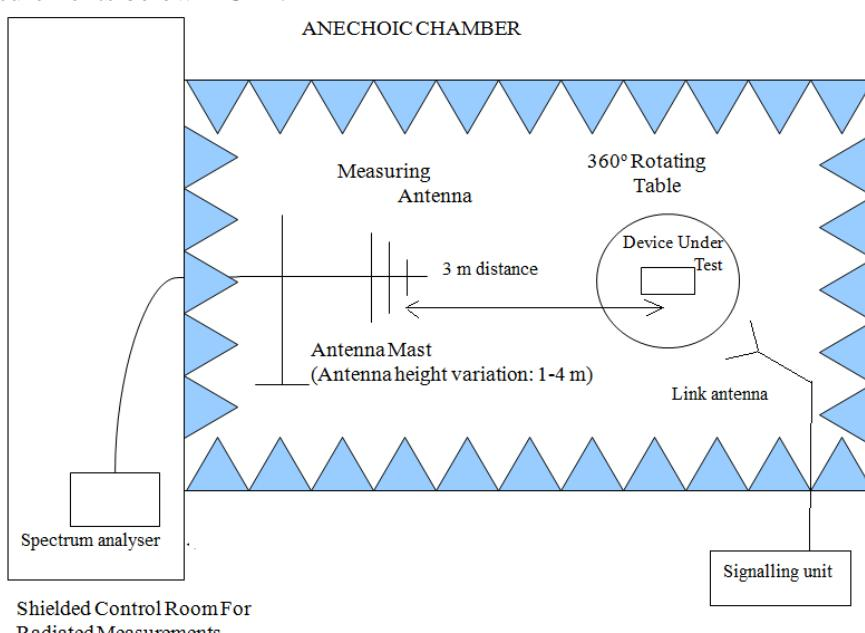
Radiated measurements above 1 GHz.
