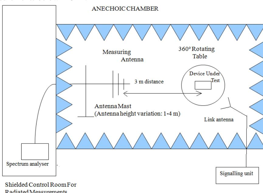
Radiated measurements above 1 GHz.
