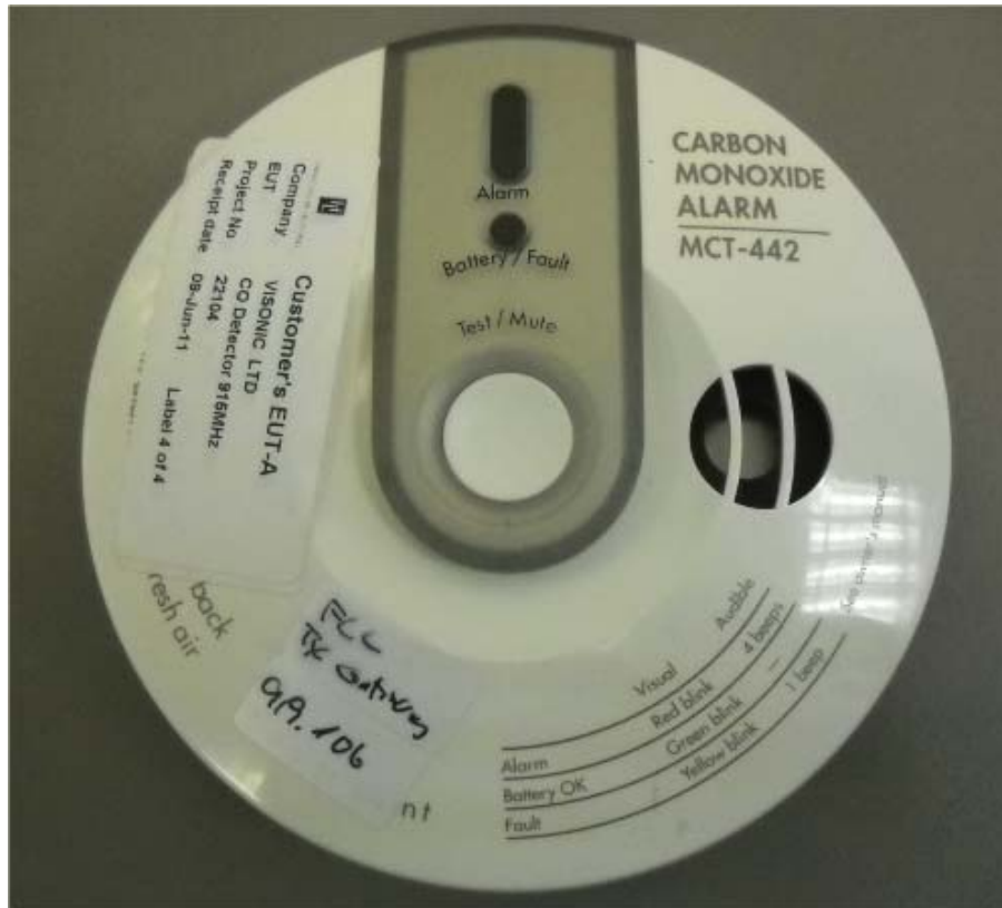
Photograph No.1 CO gas detector front view
