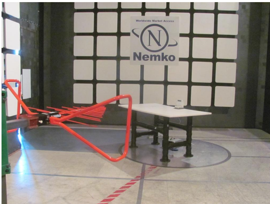
Figure 8.4-2: Transmitter output power and e.i.r.p. setup photo
