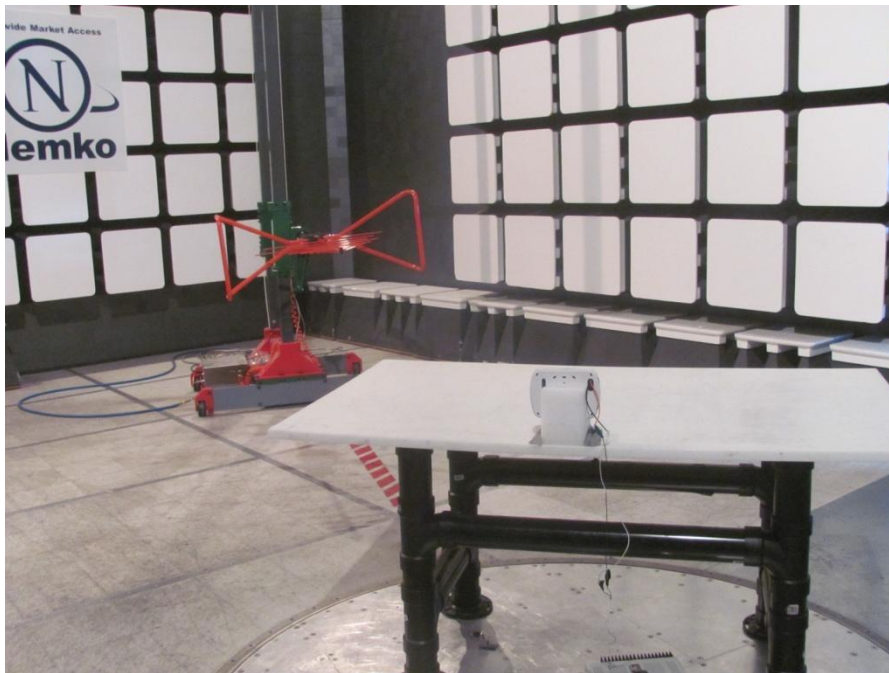
Figure 8.4-1: Transmitter output power and e.i.r.p. setup photo
