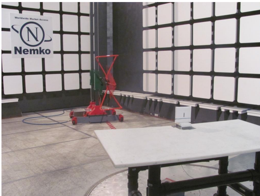
Figure 8.5-6: Spurious (out-of-band) emissions setup photo
