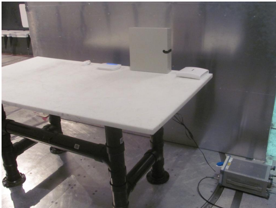
Figure 8.1-4: AC power line conducted emissions on phase setup photo
