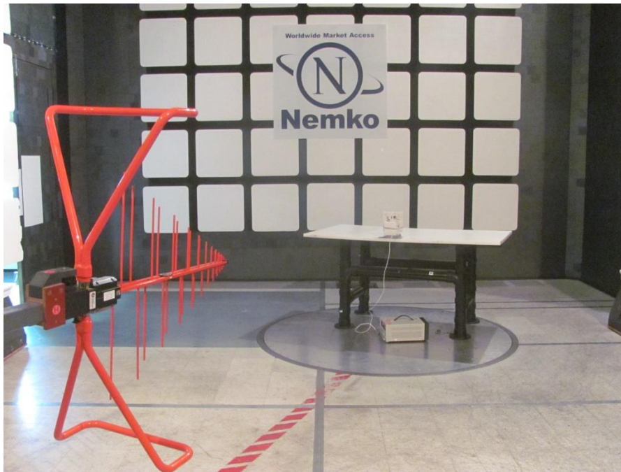
Figure 8.4-1: Transmitter output power and e.i.r.p. setup photo
