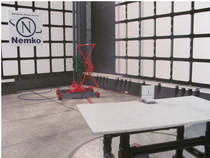
Figure 8.4-2: Transmitter output power and e.i.r.p. setup photo
